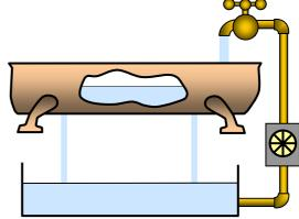
The only difference is that the pump will have to work twice as hard as before to maintain the level. It means that the rate of flow of water from the tap must be **TWICE AS GREAT** as before and energy is used by the pump at **TWICE THE RATE**.
